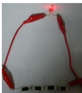
Fig. S12 Image of the 80%-PANI/GO/CNTs composite film-like supercapacitor lighted a LED.
